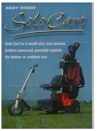
A Cork Ballington designed ride-on golf buggy with two batteries and a battery charger.
